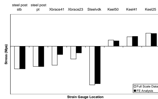
Figure 6: Comparison of FE Analysis and Full Scale Data for Asymmetric Sag Longitudinal Bending Scenario
